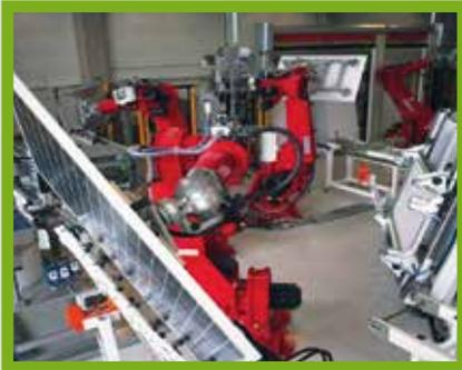
The Layup Station automatically aligns and places completed solar cell strings in position for module assembly. The Layup Station includes a string unloader robot for string transport, a string aligner, and a ball table for module layup.
