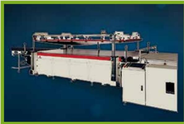
The Layup Station automatically aligns and places completed solar cell strings in position for module assembly. The Layup Station includes a string unloader robot for string transport, a string aligner, and a ball table for module layup.
