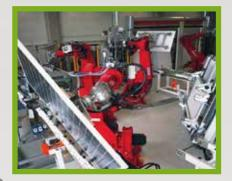
The Layup Station automatically aligns and places completed solar cell strings in position for module assembly. The Layup Station includes a string unloader robot for string transport, a string aligner, and a ball table for module layup.
